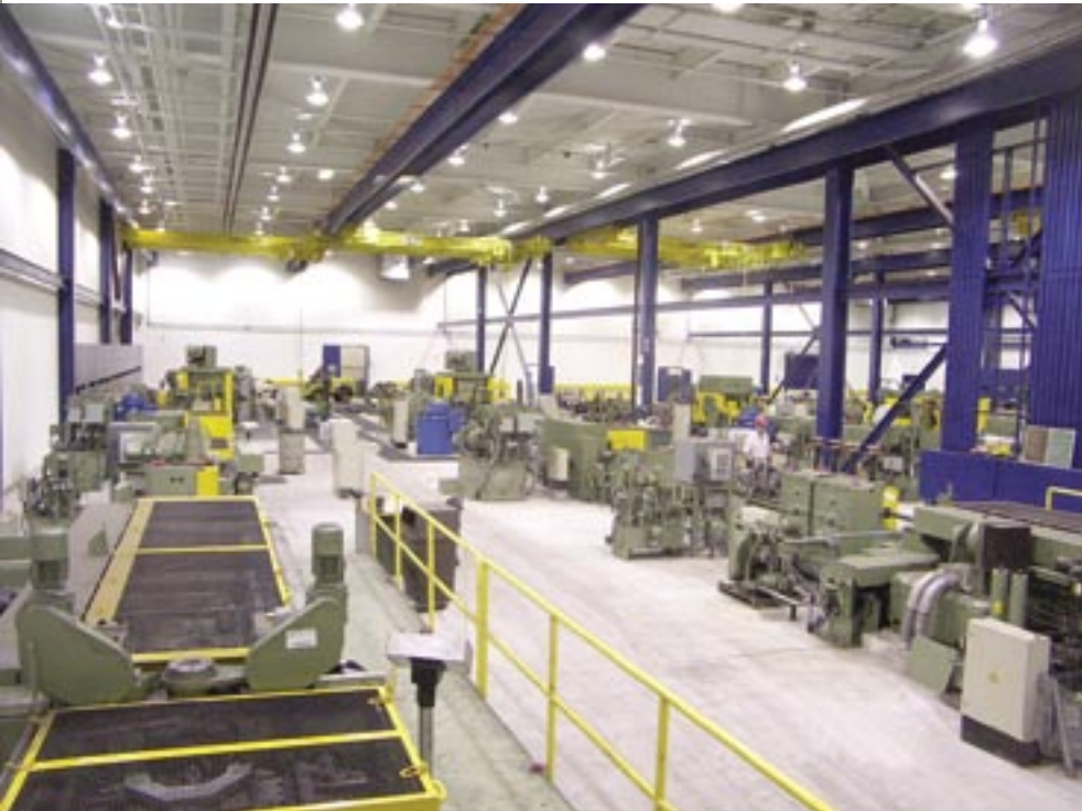
Building 18's six side-by-side cold-finishing lines are arranged in order of bar size capacity. The largest machine, seen at left, can produce 2-inch diameter bar directly from coil. ▲
