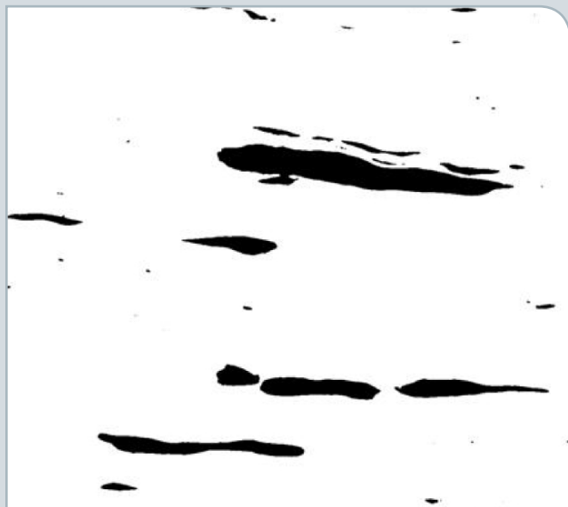
FIGURE 5 :: Elongated sulfides as they appear after hot rolling.
